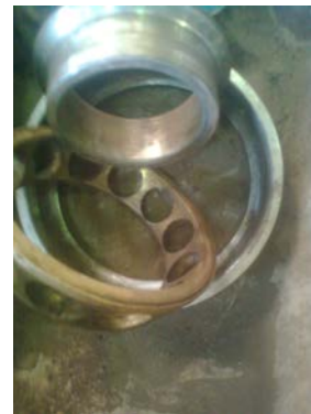
Fig.9. Damaged cage of the SKF 6228 rolling bearing
