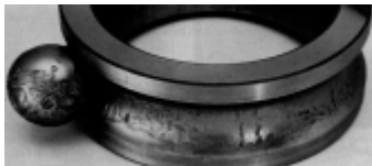
Fig.7. Damaged rolling elements of the SKF 6228 on motor
