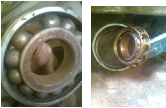
Fig.10 Damaged outer race SKF 6228 rolling bearing
