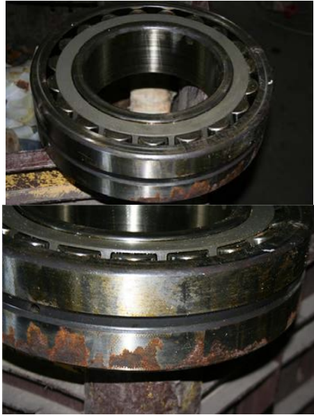
Fig.15 Damaged outer ring of bearing 22240 CC/W33
